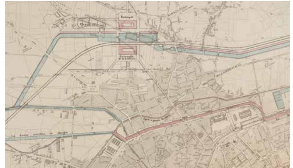
An ambitious plan (never realised) for a diversion of the Brussels-Charleroi Canal, 1864. As well as creating a new ship canal and 'seaport' in the municipality (blue), the plan would have seen the Senne, Petite Senne and part of the existing canal disappear to make way for boulevards (red). (© KBR)
