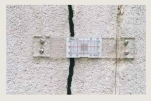
Installation of crack measuring apparatus in different areas following the schedules of condition and the observation of the presence of cracks. The image shows the façade of *Le Cerf/ De Heert*. Euville stone ( $\odot$  HHU, 2000).
