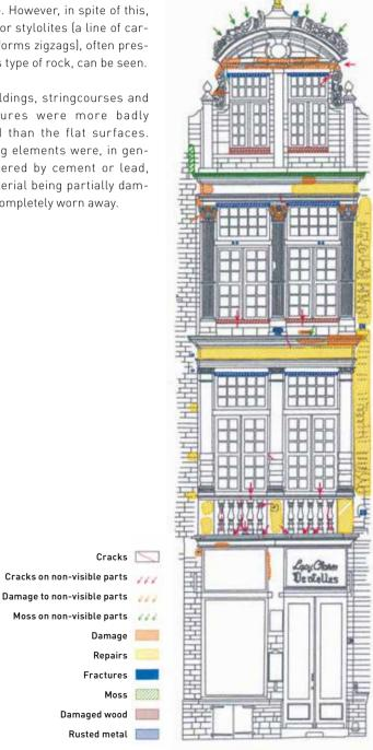
L'Âne/Den Ezel. Sketching of façades with survey of pathologies. This survey was supplemented with photographs and descriptions of each damaged element (© HHU, 2000).
