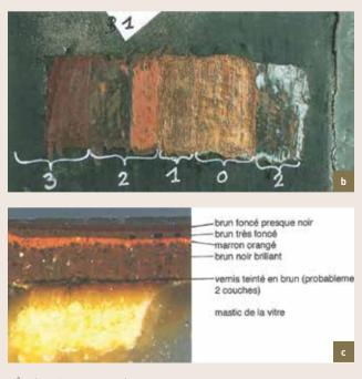
L'Âne/Den Ezel. a, b and c) Stratigraphic sampling and macro photography of a window frame indicating an original layer of varnish (a and b) © M. Decroly, 2002; c) © KIK-IRPA, 2002).
