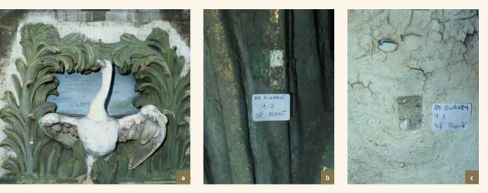
Le Cygne/De Swane. Stratigraphic sampling on the swan. a) General view of the swan with location of sampling; b) Sampling in the foliage; c) Sampling in the plumage (© L. De Clercq, 2004).
