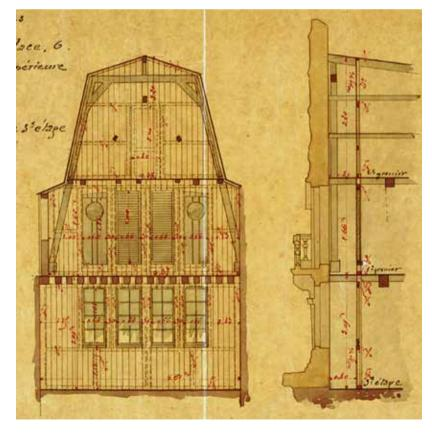
Le Cornet/Den Horen. Example of installation of temporary interior partitions on the 3<sup>rd</sup> floor and the attics. Plan dating from 15 January 1901 (© AVB).
